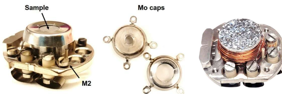
Figure 12. Elmitec sample holder with the cap mounted is shown on the left. Caps with different sizes of openings are shown in the center. The magnetic sample holder is shown on the right.
