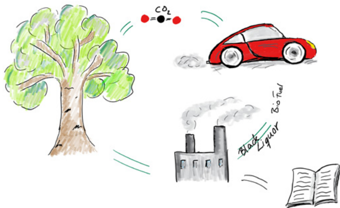
Figure 1. Lignin is a byproduct from the pulp and paper industry and can be converted into biofuel, by the use of catalytic hydrotreatment.
