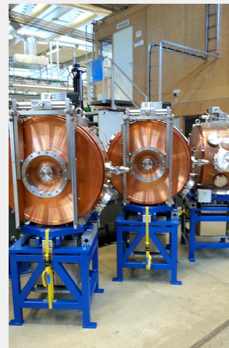
Cavities waiting to be installed in the 3 GeV ring at MAX IV.
