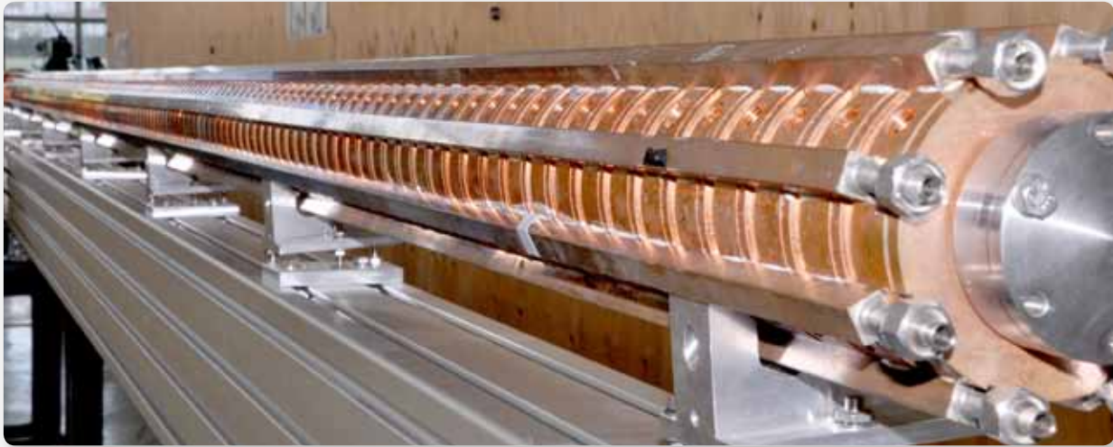
Figure 3. A five-meter long prototype segment for the MAX IV linac.
