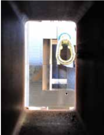
A magnet block for the 3 GeV ring as seen through a magnet block dummy.
