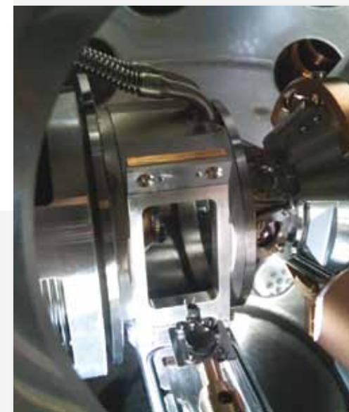
Figure 5. The high pressure cell in the APXPS instrument.
