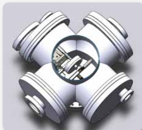
Figure 3. The HHG gas jet chamber.
