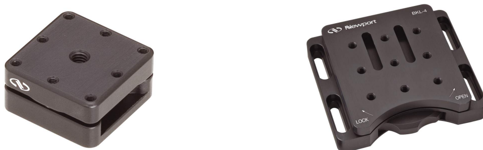
Figure 44 Kinematic bases for smaller sample environments. Left: Newport BK-1A-B, 25.4x25.4 mm 2 , magnetic base. Right: Newport M-BKL-4, 88.9 x 101.6 mm 2 , with locking thread. Photo credit: www.Newport.com .
