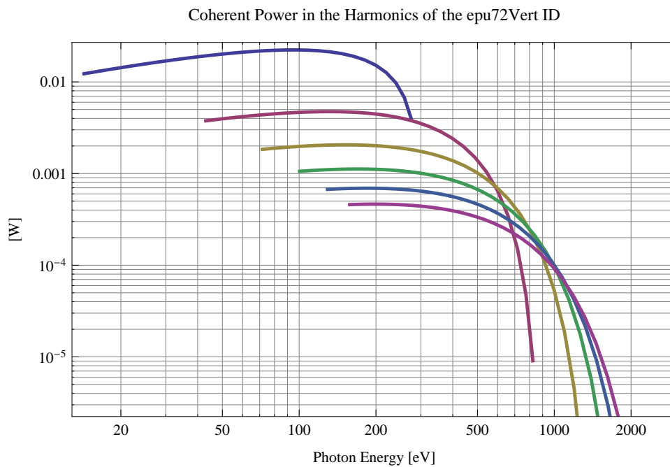
Figure 293: The power of coherent synchrotron radiation in the harmonics of the epu72Vert
