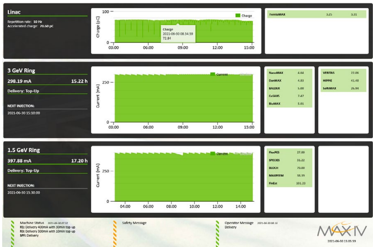
Figure 1: Screenshot of the MAX IV Status page on June 30 th showing delivery at 300 mA top-up in the 3 GeV ring. It also shows the concurrent delivery of 400 mA in top-up for the 1.5 GeV ring and 10 Hz operation of SPF.
